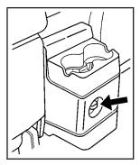
Put the cover in position and insert and tighten the wing nut to secure it.
